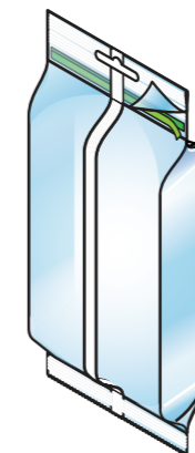
F 05 confezione a cuscino con euro slot e cross web zip pillow bag with gusset, euro hole punch and zip cross web material
